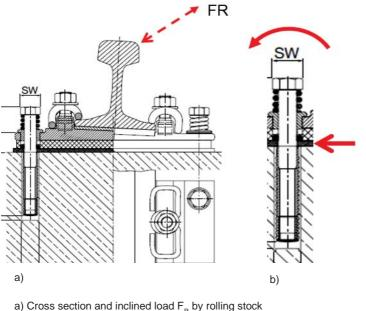
b) Cantilever bending of Hilti direct fixation fasteners by means of shear force and moment
